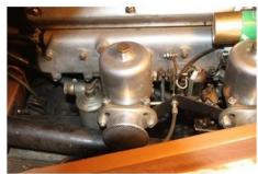
Going to three SUs and in particular three Webers is going to increase the fuel consumption and that means the fuel pump working harder. Fitting a high pressure pump is the answer. Lastly, tempting as it is to have bell mouth intakes sticking out of your carburettors, if that is your choice, at least fit ones with metal gauze over them to reduce the rubbish that gets sucked into the engine.
