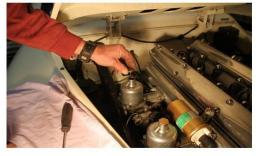
with two 2 in sandcast H8 SUs and these were later offered as a factory option on 140s. For this conversion, the inlet manifold was simply a standard item with the porting enlarged to 2 in. Various variations in inlet manifold and filters were used, including differences between Left and Right Hand Drive models. There were also several variations on the starting carburettors, their fitment and location.
