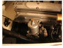
Unless you have them, going from two 1% in to two 2 in SUs, with the enlargement of the inlet manifold ports, is the first step. This is relatively easy and cost effective. However remember that any tuning will increase the stresses in the engine so be cautious if your engine is a bit tired.
