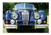
Jaguar XK140's have a level of sophistication compared to the earlier XK120. Re-designed to include rack and pinion steering, telescopic shock absorber damping to the rear, an overdrive gearbox option along with a more powerful engine and uprated to 2 inch carburettors.
