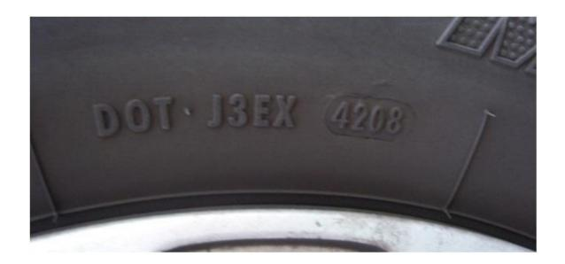
Here the relevant numbers are 4208. These digits tell you that this tyre was made in the  $\underline{42}$ nd week of  $\underline{2008}$ . Tyres made before 2000 may have only a three number code. Such a tyre marked 408 would refer to a maker's date of the  $\underline{40}$ th week of the  $\underline{8}$ th year in the decade so it could be 1998, 1988 or earlier.
