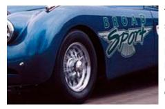
The main advantages of wire wheels were that they were stronger and helped brake cooling. An advantage if you were racing was that wheel changes were faster. They were also lighter meaning less un-sprung weight, which helped roadholding. Above all they looked smarter and sportier. The disadvantages are that they are pigs to keep clean, spokes can come loose or break and the splines wear.
