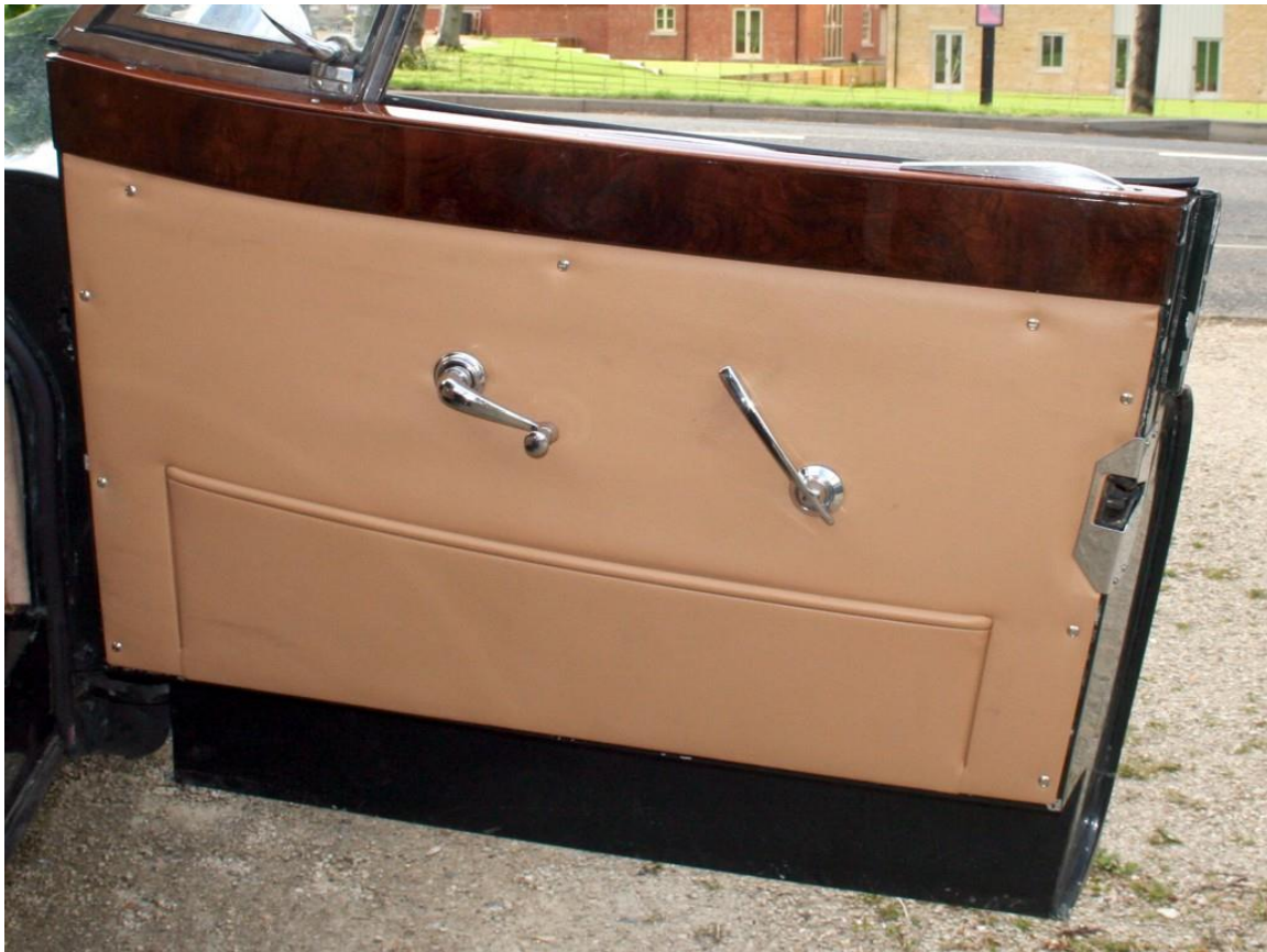
The door panel fitted, showing the door pocket, which is as the panel is supplied.
