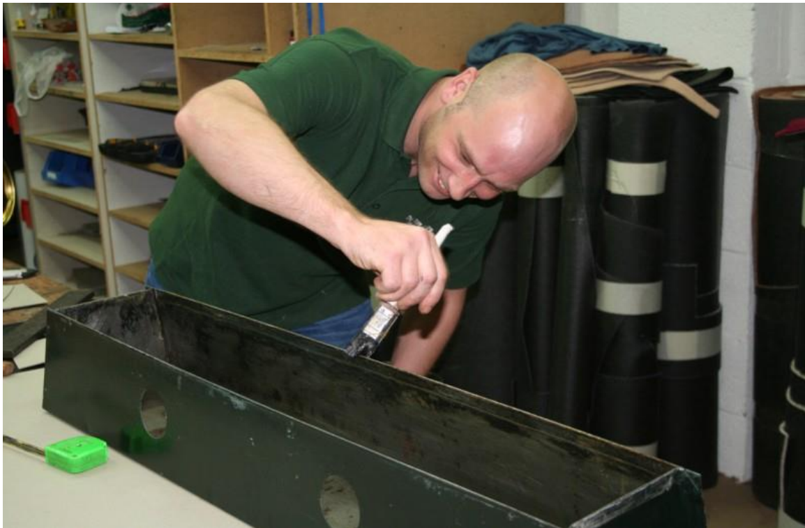
The adhesive being brushed on to the storage box.
