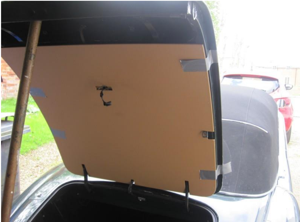
The boot panel held in place with tape to keep it place before drilling the screw holes.
