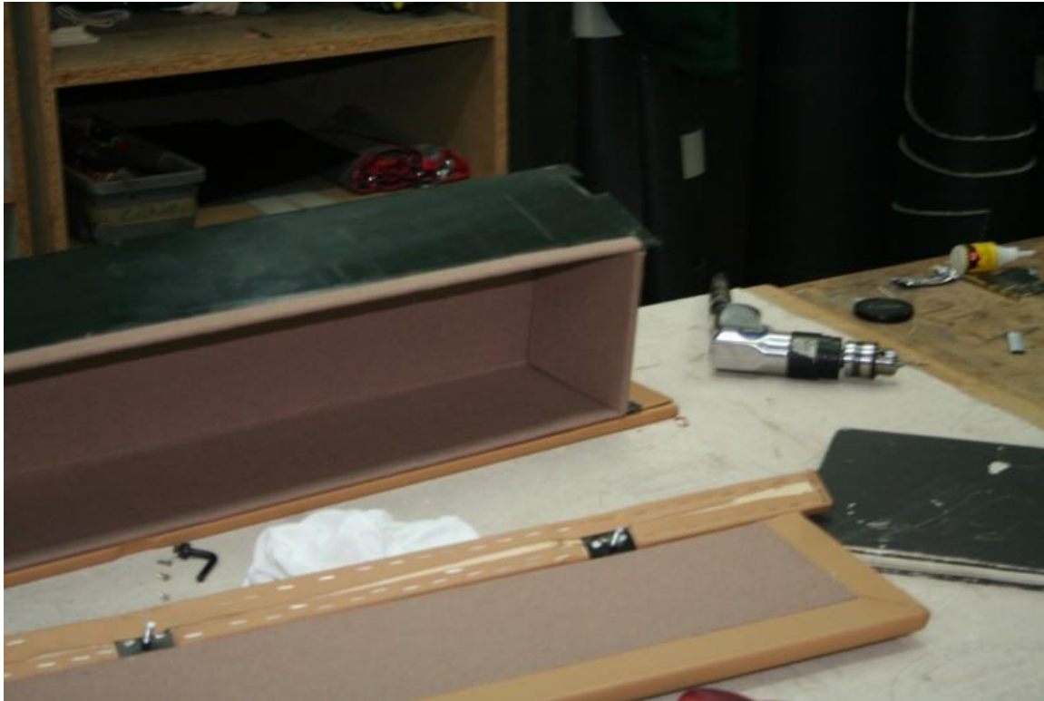
This shows the box with the cloth interior and lid with the leather cloth covering and cloth section.
