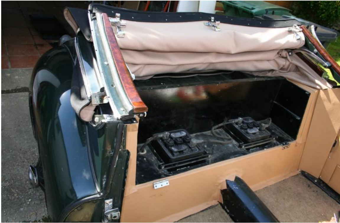
Here the leather-cloth covering of the rear interior bodywork is seen prior to fitting the storage box.
