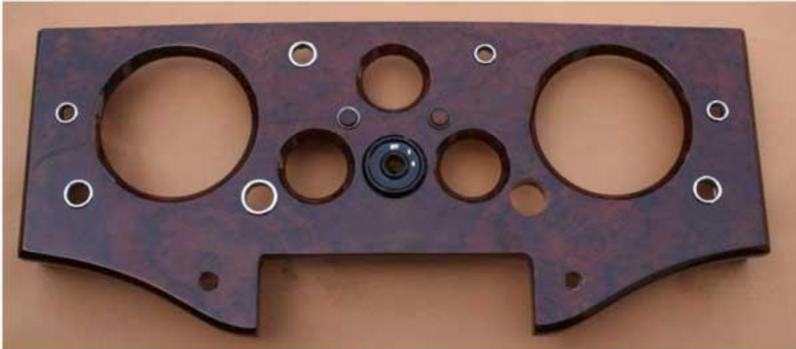
The refurbished dash with the switch escutcheons and warning lights fitted
