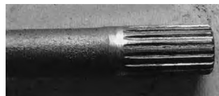
Chattering on half shaft splines.
