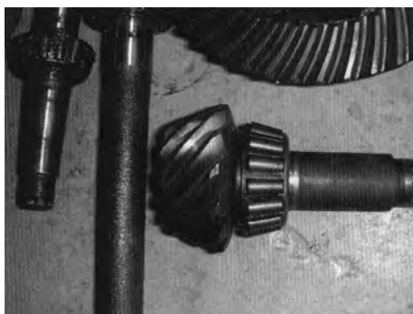
Worn crown wheel and pinion.
